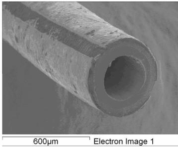
Fig. 4. a) SEM image of the catheter coated with polypyrrole and micromachined into two polymer electrodes.
