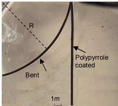
Fig.5. Experimental result showing the catheter at two states: initial, bent.
