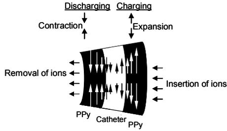
Fig. 3. Stress distribution upon insertion and removal of ions from the polypyrrole layer.
