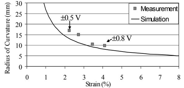
Fig. 6. Experimental and simulated bending radius versus strain for  $40 \mu\text{m}$  thick polymer
