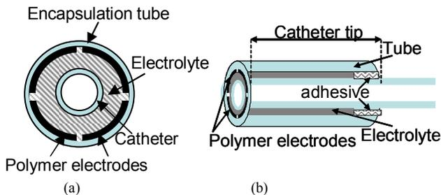
Fig. 7. Encapsulated design for active catheterization application: a) cross section view, b) side view.
