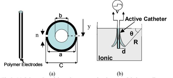
Fig 2. (a) Schematics of the polymer coated catheter modeled as a trilayer, (b) Actuation of the trilayer by applying voltage inside an electrolyte
