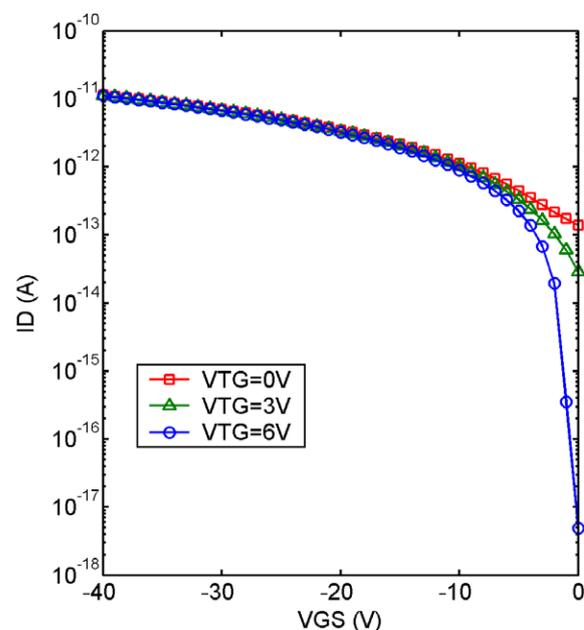
Fig. 10. The transverse characteristics of the simulated 200 nm dual gate OFET at different top gate biases ( $V_{DS} = -0.5$  V).
