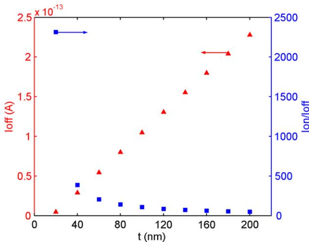
Fig. 8. The variation of the off current and the on/off current ratio in the OFETs with the semiconductor thickness ( $V_{DS} = -0.5$  V).
