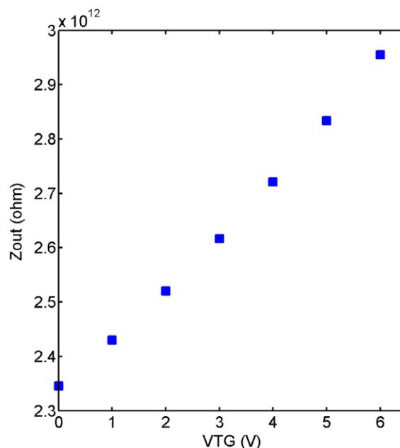
Fig. 13. The variation of the output impedance in the 200 nm thick dual gate OFET with the top gate voltage ( $-60 < V_{DS} < -40$  V and  $V_{GS} = -40$  V).
