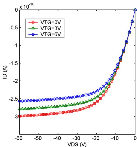
Fig. 12. The output characteristics of the simulated 200 nm dual gate OFET in different biases of the top gate ( $V_{GS} = -40$  V).
