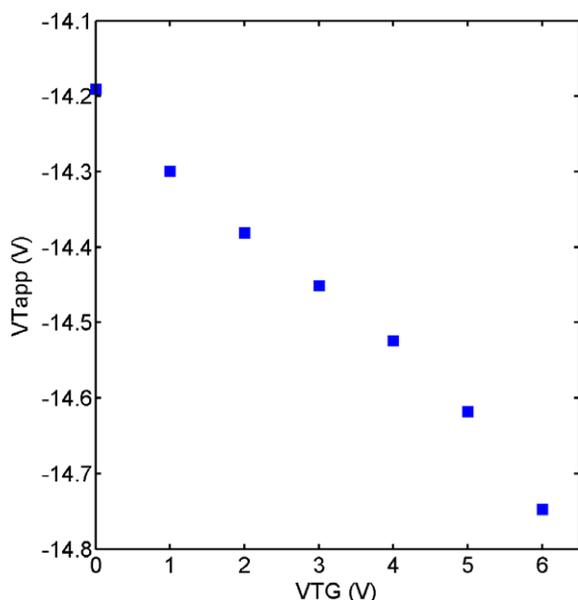
Fig. 11. The variation of the apparent threshold voltage in the 200 nm thick dual gate OFET with the top gate voltage ( $V_{DS} = -0.5$  V and  $V_{GS} = -40$  V).
