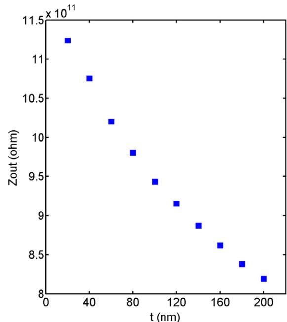
Fig. 7. The variation of the output impedance in the OFETs with the semiconductor thickness ( $-60$  V  $< V_{DS} < -40$  V and  $V_{GS} = -40$  V).
