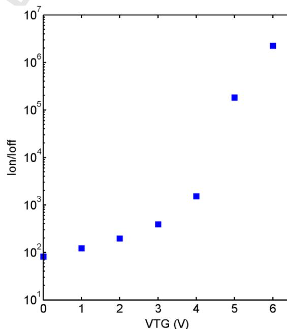
Fig. 14. The variation of the on/off current ratio in the 200 nm thick dual gate OFET with the top gate voltage ( $V_{DS} = -0.5$  V).
