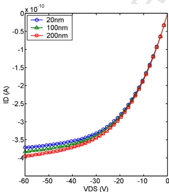
Fig. 6. The output characteristics of the OFETs with the different semiconductor thicknesses ( $V_{GS} = -40$  V).
