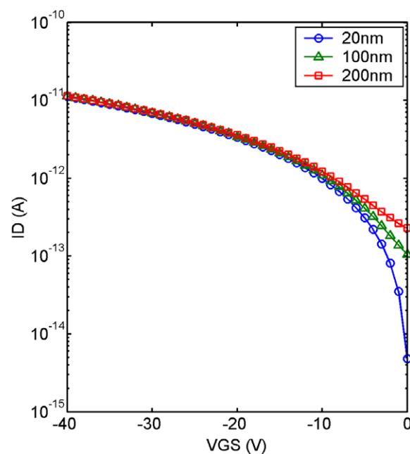
Fig. 4. The transverse characteristics of the simulated OFETs with the different semiconductor thicknesses ( $V_{\text{DS}} = -0.5 \text{ V}$ ).
