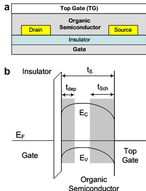
Fig. 3. (a) A schematic of a dual gate OFET and (b) the energy band diagram at the both gate interfaces (equilibrium condition -  $V_{GS} = V_{TG} = 0$  V).
