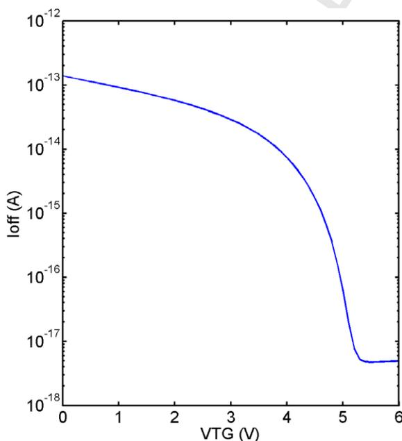
Fig. 9. The variation of the off current in the 200 nm thick dual gate OFET with the top gate voltage ( $V_{DS} = -0.5$  V and  $V_{GS} = 0$  V).
