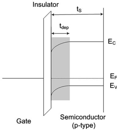
Fig. 2. The energy band diagram for a MIS device at the equilibrium ( $V_{GS} = 0$ ).
