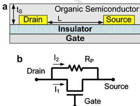
Fig. 1. (a) A schematic of a bottom contact OFET and (b) a simple model for the device consisted of an ideal IGFET and a parallel resistor.
