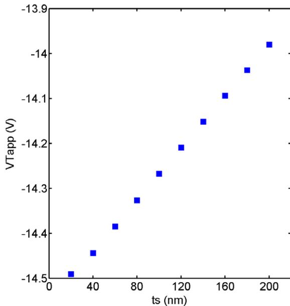
Fig. 5. The variation of  $V_{Tapp}$  in the OFETs with the semiconductor thickness ( $V_{DS} = -0.5$  V).
