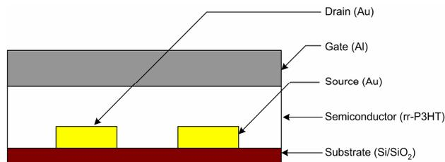
Fig. 1. OMESFET structure. Horizontal dimensions are not to scale.
